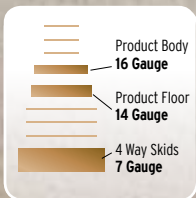
STEEL GAUGE CONSTRUCTION
